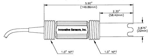
The Model 17 is a combination pH sensor designed for insertable use in process and waste water applications where greater pipeline penetration is required.
